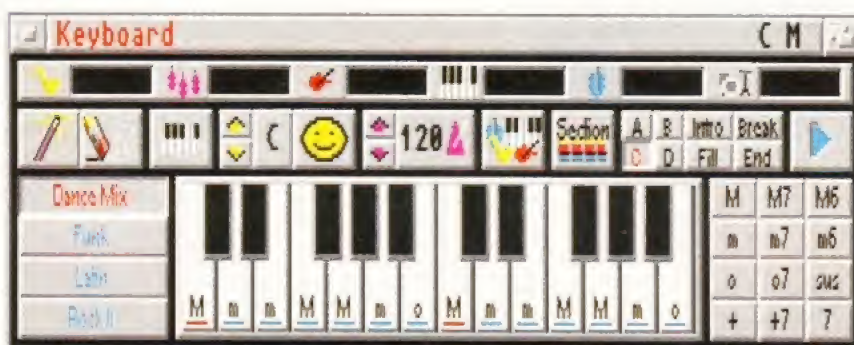
The keyboard window of SuperJAM! is the main control centre for the program. From here you can call up styles, play chords and melodies, and access all the detailed editing windows.
